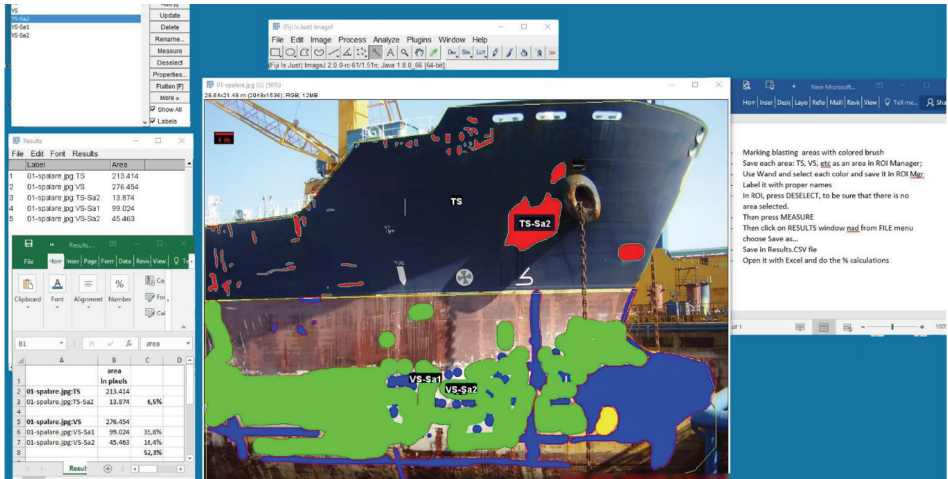
FIGURE 5 Determining blasting percentages after indocking inspection.
