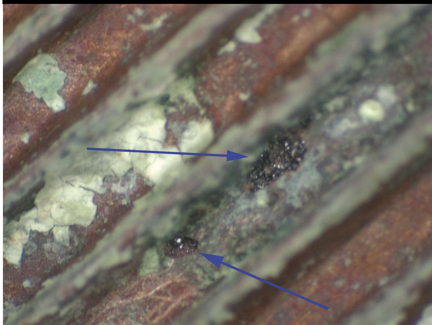
Pitting beneath internal diameter (ID) deposits, 30X original magnification.
